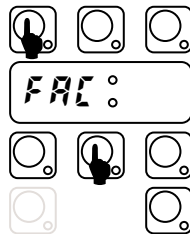
Fig. 5 Enter into Factory Parameters (Hold down buttons for at least five seconds)..
